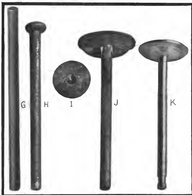
Fig. 2—Components of the built-up valve, showing the various stages of development of valve stems and mushroom welded to it
